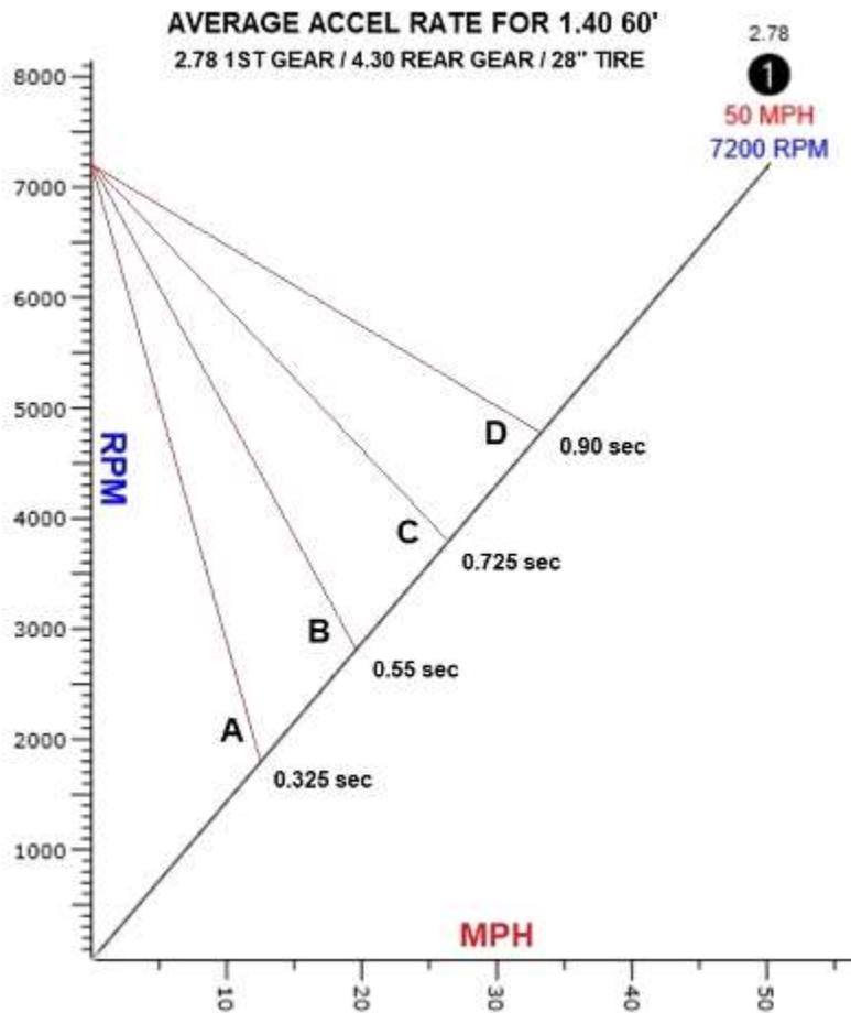
In the graph above, lines A,B,C, and D represent different rates that the clutch is pulling down a 600ft/lb
